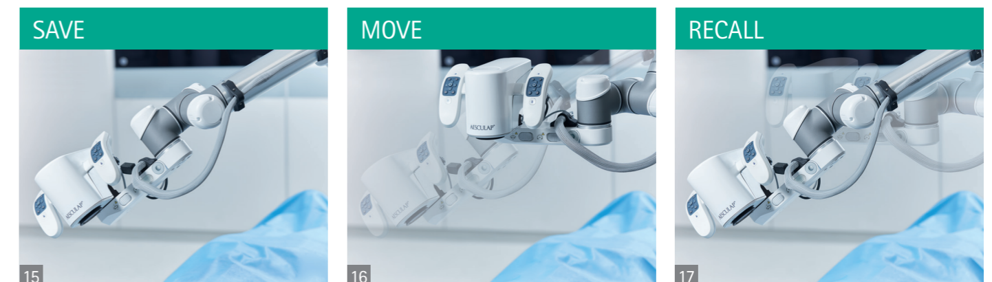
Fig. 15-17: Waypoints: Seamlessly return to a previously saved location, including zoom and focus
