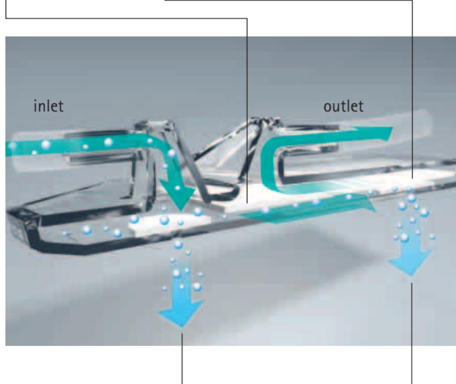
B. Braun infusion filters prevent air embolism by two 0.02 µm hydrophobic Polytetrafluoroethylene (PTFE) membranes. They allow for reliable air venting regardless of filter position during application.
