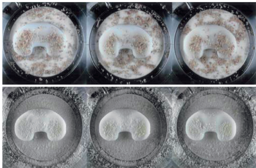
Fig. 2 ▲ Sample chamber heavily contaminated with cortical bone (above) and bone cement (below) to simulate wear on the multilayer system under extreme wear conditions
